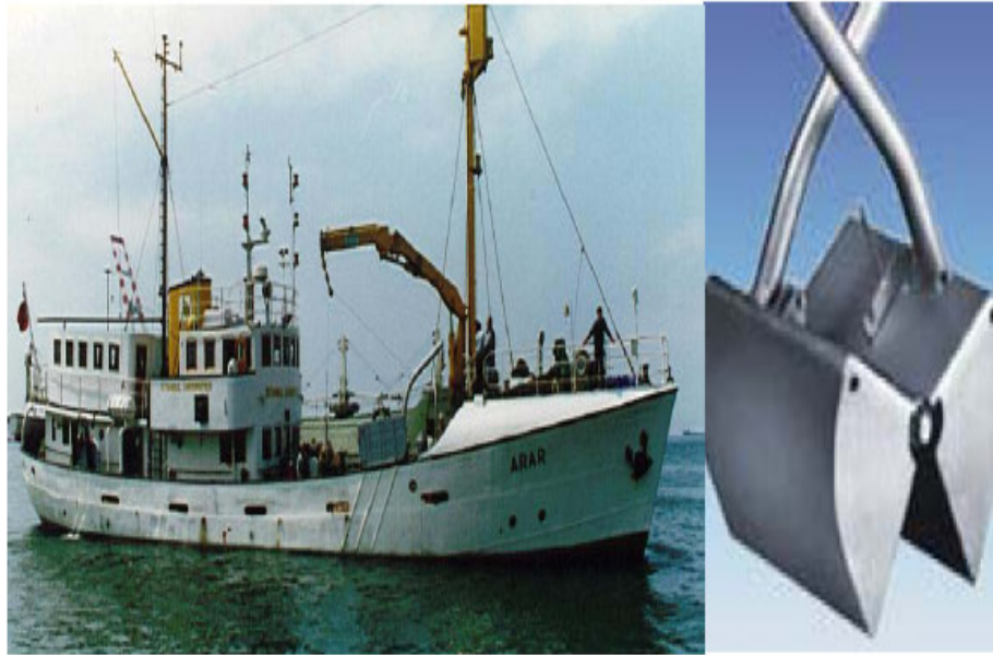
Figure 3. 2. The research ship, ARAR, of İstanbul University and Van Ween grab sampler
