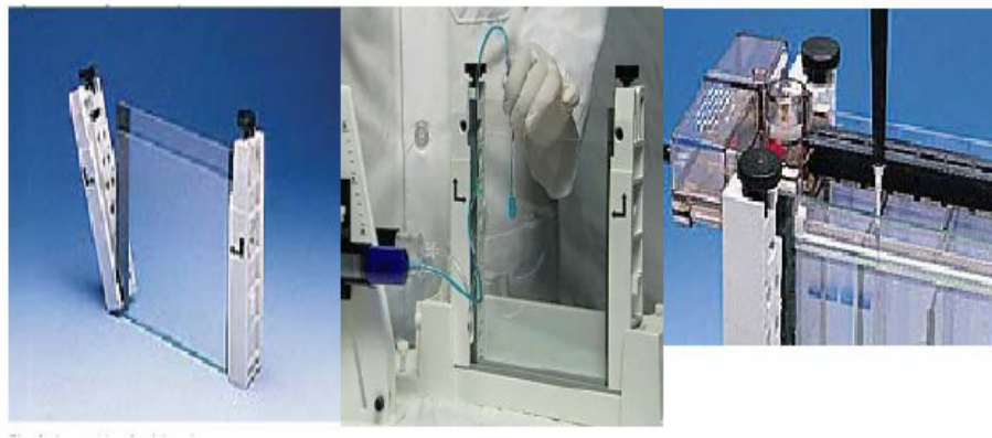
Figure 3. 4. Assembling and loading of perpendicular gradient gel sandwich
