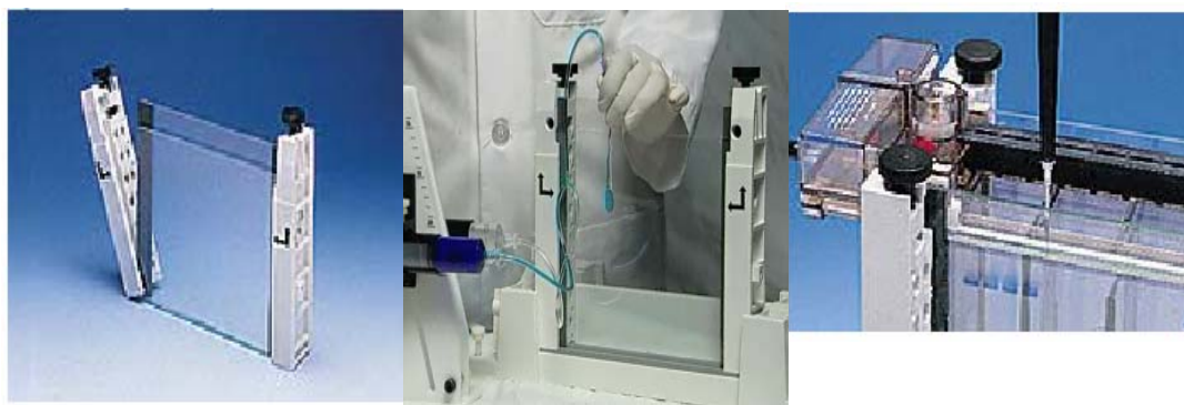
Figure 5.4. Assembling and loading of perpendicular gradient gel sandwich
