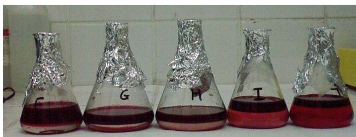
Figure 3.29. The phase separations of toluene(7)-water(3) with varying ethanol additions at 20°C.
