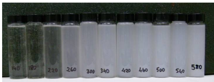
Figure 5.3. The samples collected during flushing with 20% ethanol solution at 40 0 C (low flow rate).
