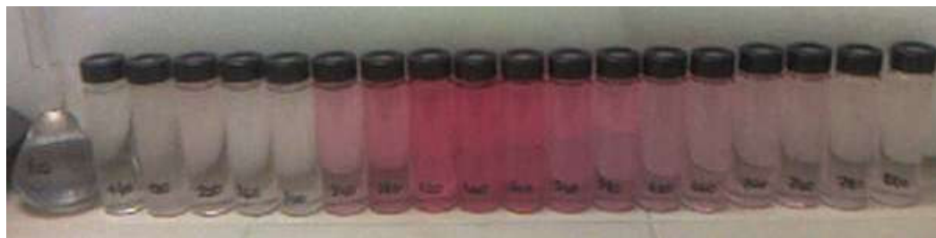
Figure 4.25. The samples collected during flushing with 40% ethanol solution at intermittent flow rate (20°C).
