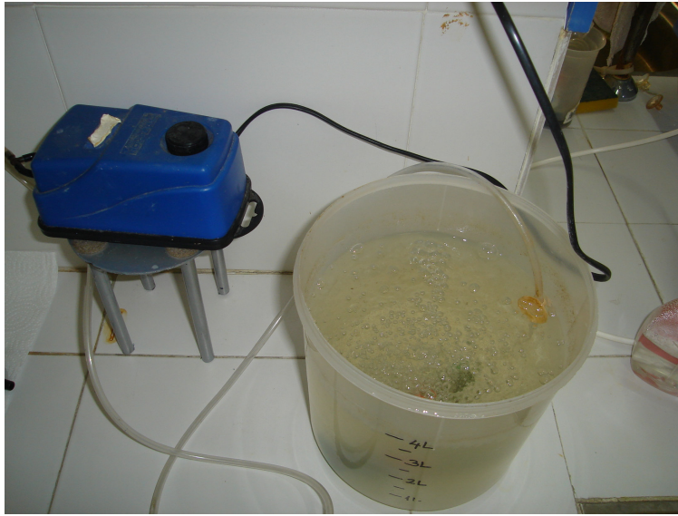
Figure 4.3 Batch reactor used to enrich the microorganisms in Ömerli water
