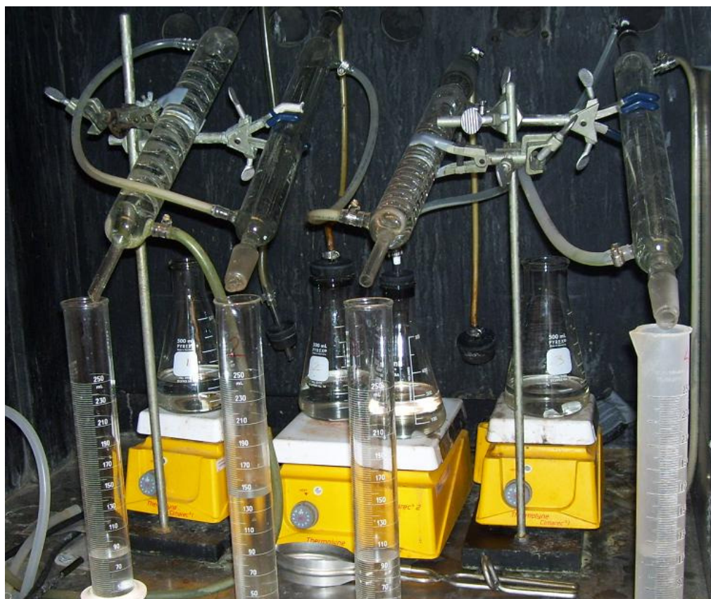
Figure 4.5. Distillation setup for VFA analysis
