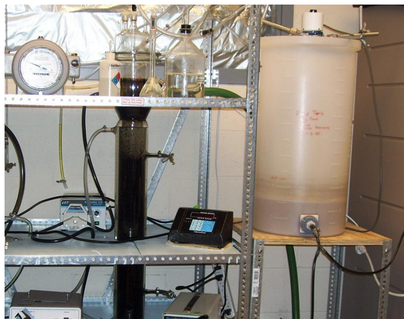
Figure 5.2. Experimental setup picture of the UASB reactor
