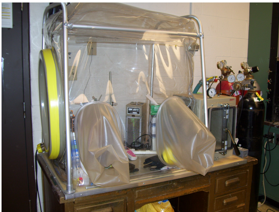
Figure 4.7. Anaerobic hood used for the MAT analysis
