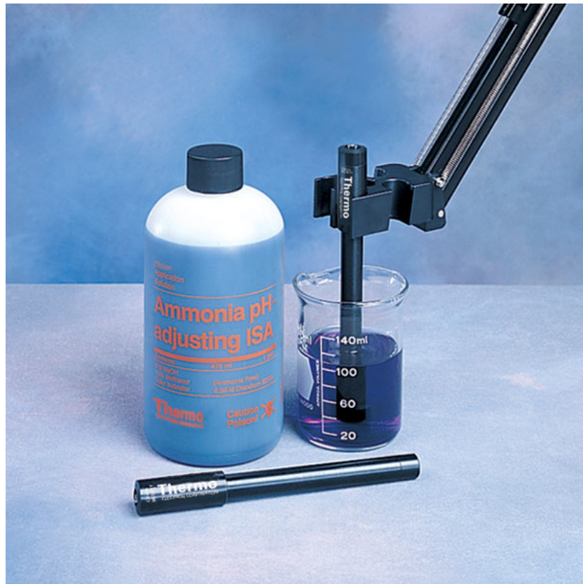
Figure 4.6. The electrode and the pH adjusting solution used in total ammonia analysis
