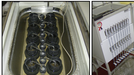
Figure 2.3. Soil permeability measurement instrument
