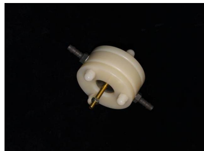
Figure 4.3. Treatment chamber of PEF generator
