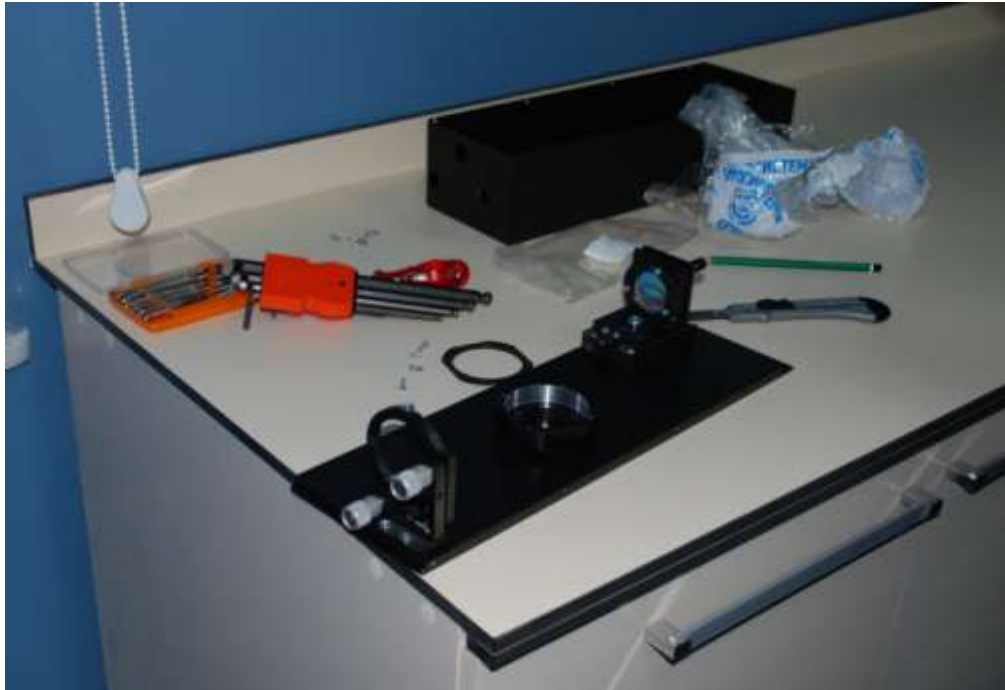
Figure C.3. Assembling the off axis collimator
