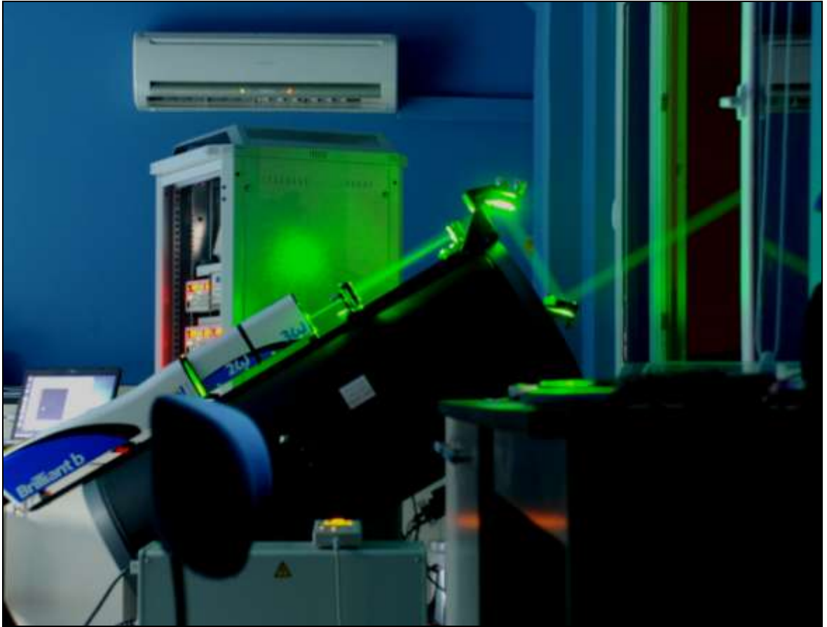
Figure B.2. The Multiwavelength Mie-Raman lidar system at TUBITAK MRC, Laser Spectroscopy Laboratory.
