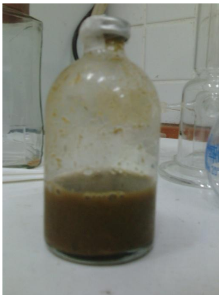
Figure 3.1. 120 mL serum bottle with 40 mL active volume used for manure slurry.
