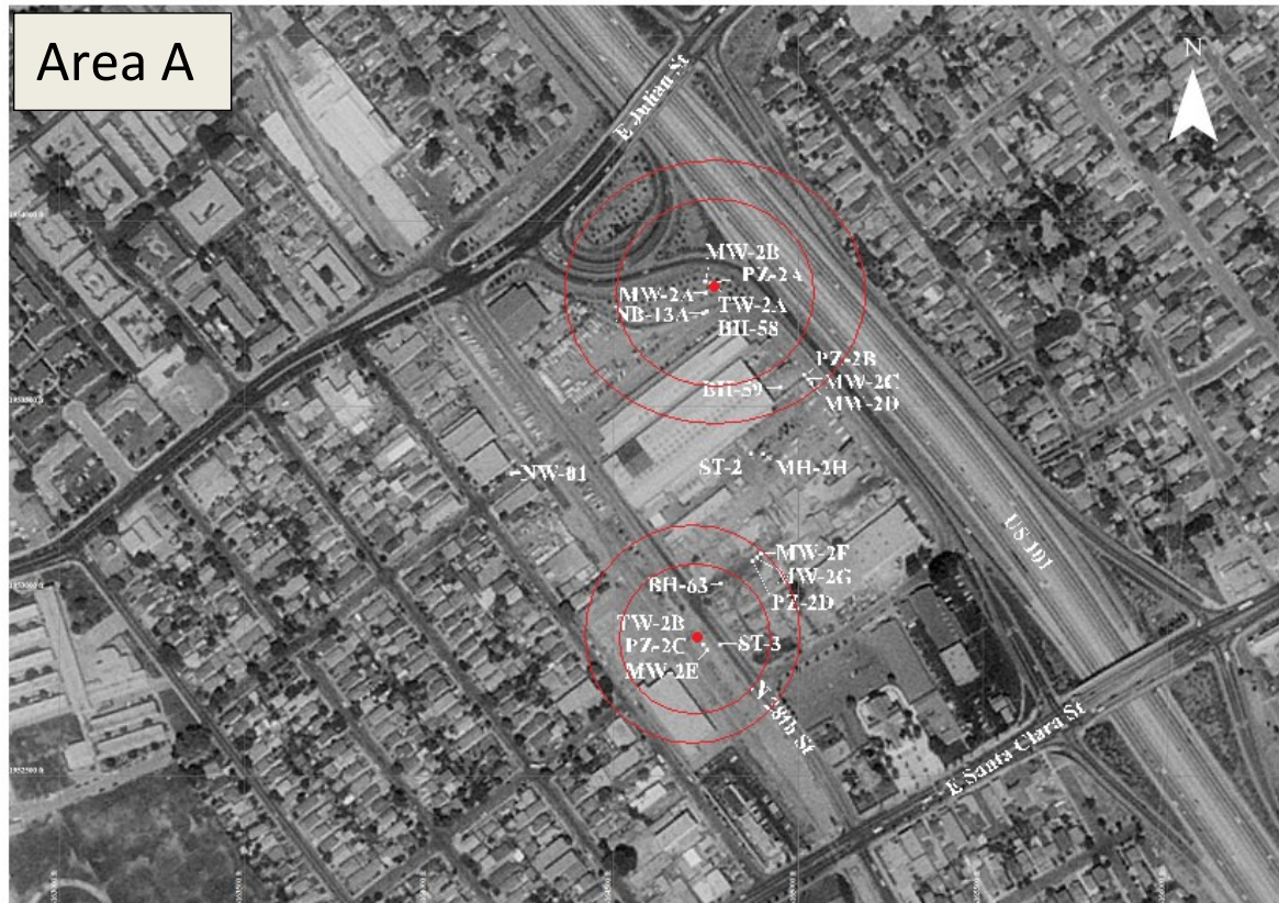
Figure 6.1. Research A showing the location of test wells, monitoring wells, boreholes and piezometers. (Source of USGS Aerial Digital Orthophoto Quadrangles: Terraserver-USA.com)
