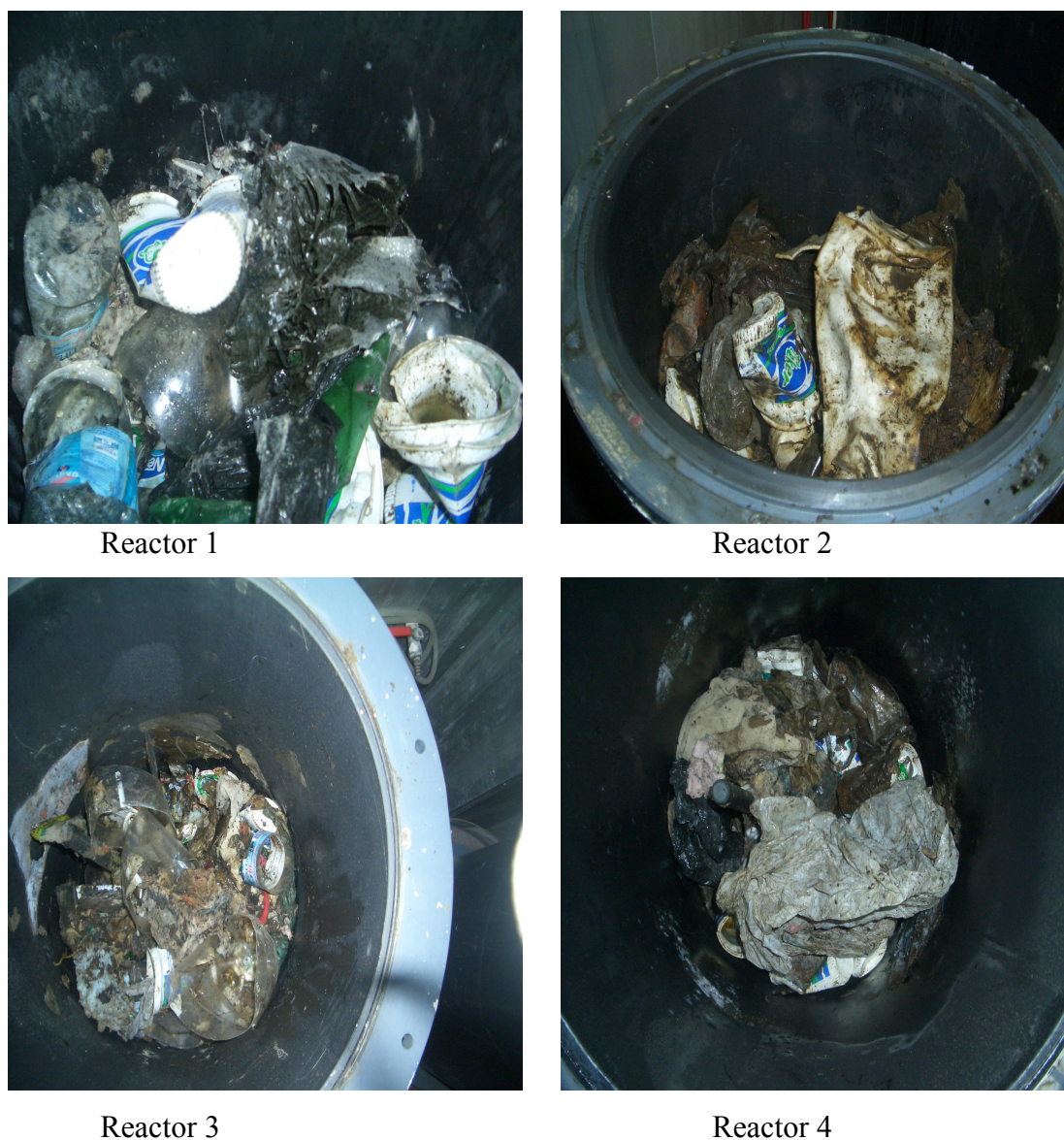
Figure 5.69. Visual observations of the settlement in the Reactors 1,2,3 and 4
