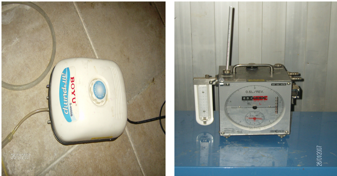
Figure 4.4. Air pump and wet gasmeter used for the reactors
