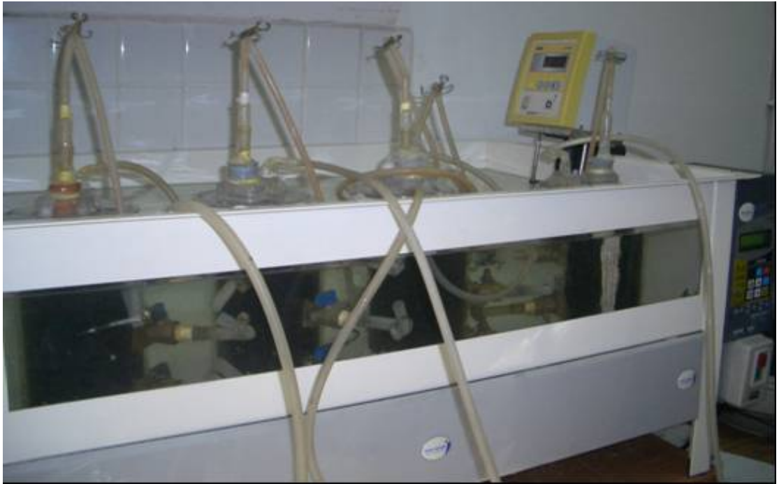
Figure 4.2. Photographic view of ASBRs
