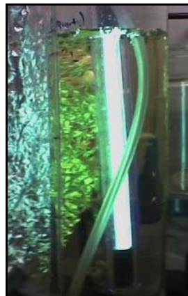
Figure 4.7. Photograph of O_3 /UV reactor.
