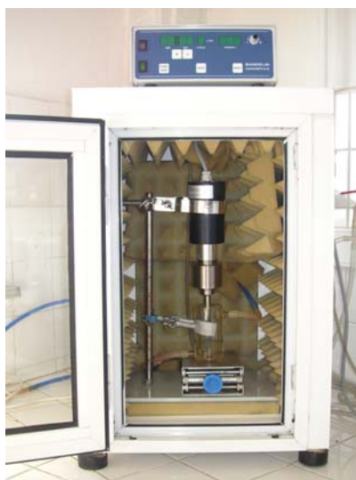
Figure 4.2. Photographic view of US1 (20 kHz probe type reactor).
