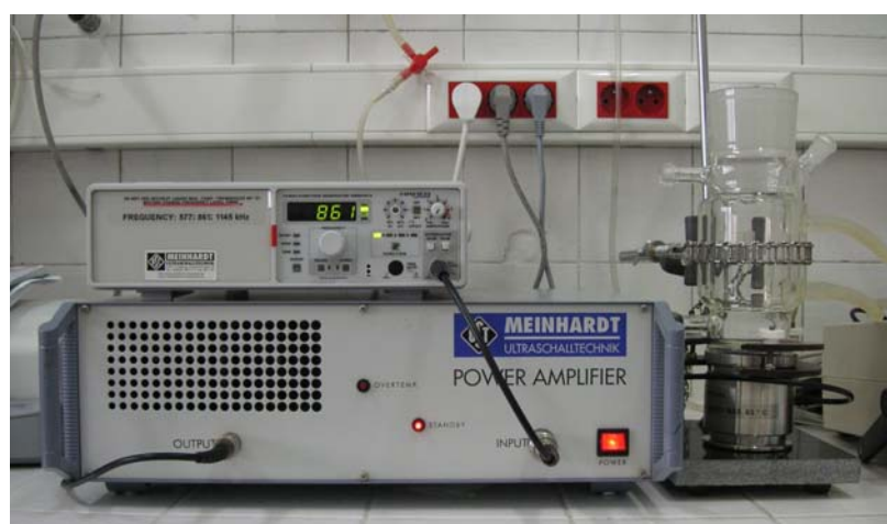
Figure 4.4. Photographic view of US3 (multi-frequency plate type reactor).
