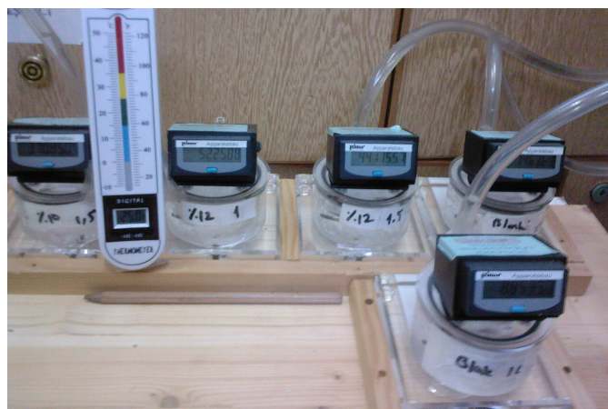
Figure 3.3. Miligascounter ® (MGC) used for the measurement of gas volume
