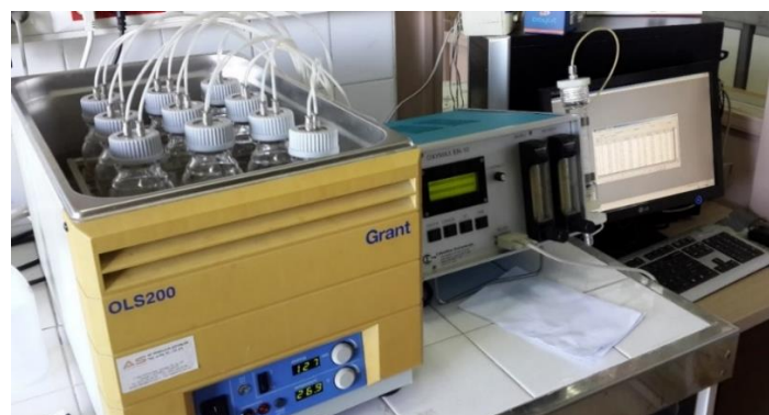
Figure 3.6. Configuration of Respirometric Test.
