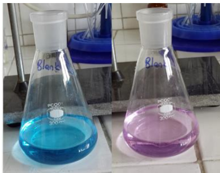
Figure 3.2. Color change in the blank before and after titration.
