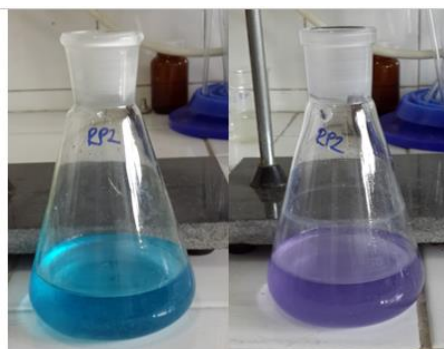
Figure 3.3. Color change in the sample before and after titration.
