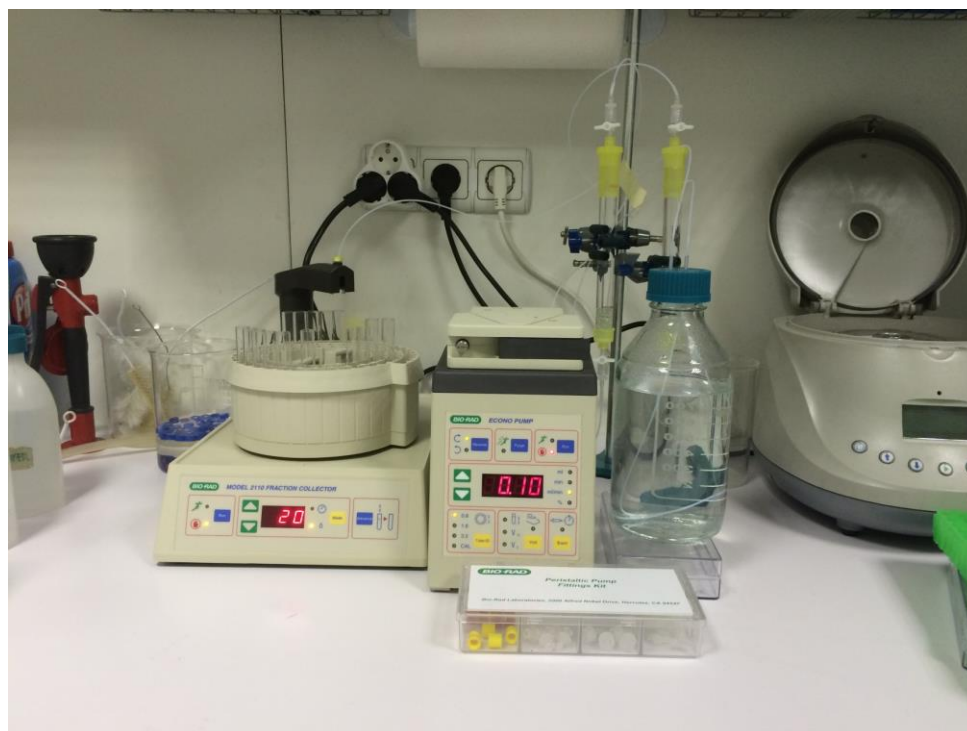
Figure 4.3: Schematic representation (upper) and actual photo (below) of packed-bed reactor setup
