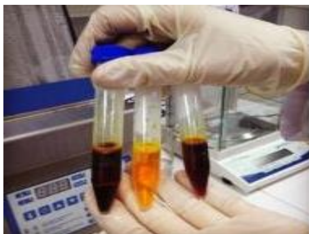
Figure 6.5. The color development after addition of DNS reagent to the assay tubes.
