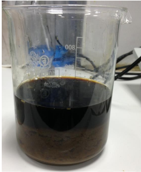
Figure 3.5. Lignin precipitation from black liquor.
