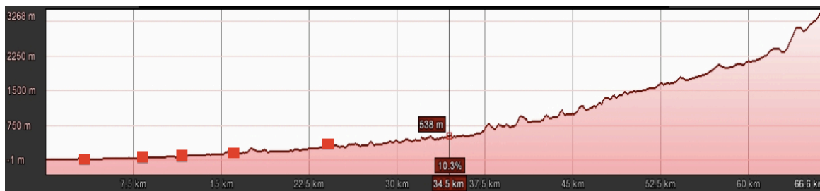
Figure 3.14. The longitudinal section of the İkizdere River with the location of the power plant of the İkizdere HES. The approximate locations of the other five power plants are plotted to the original figure. Source: Yurtseven, 2012, pp. 134, Ek Şekil 32.
