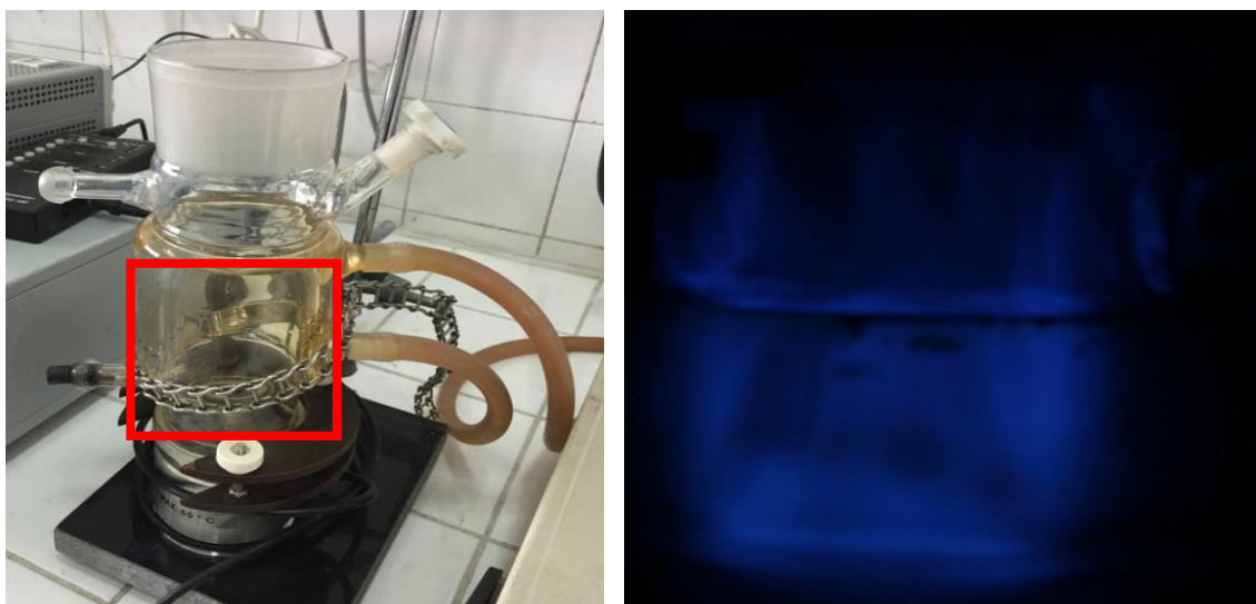
Figure 3.8. The image of sonochemiluminescence in luminol solution (250 mL) at R4 reactor ( f=861 kHz).
