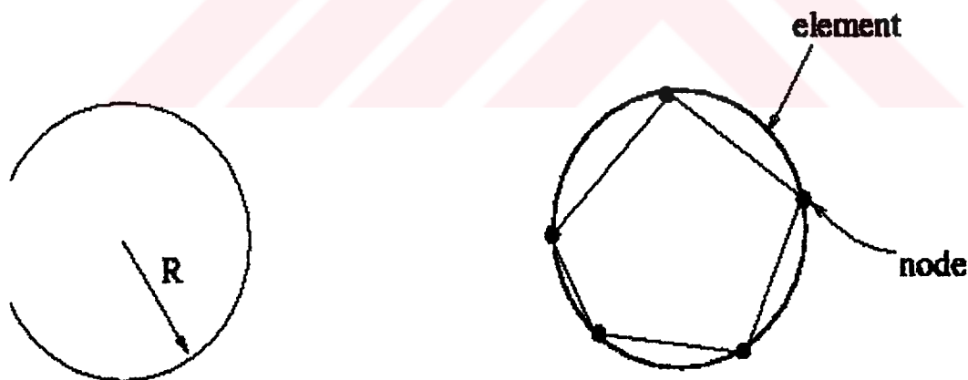
Figure 3.1 Circle discretized into 5 "elements" and 5 "nodes"
