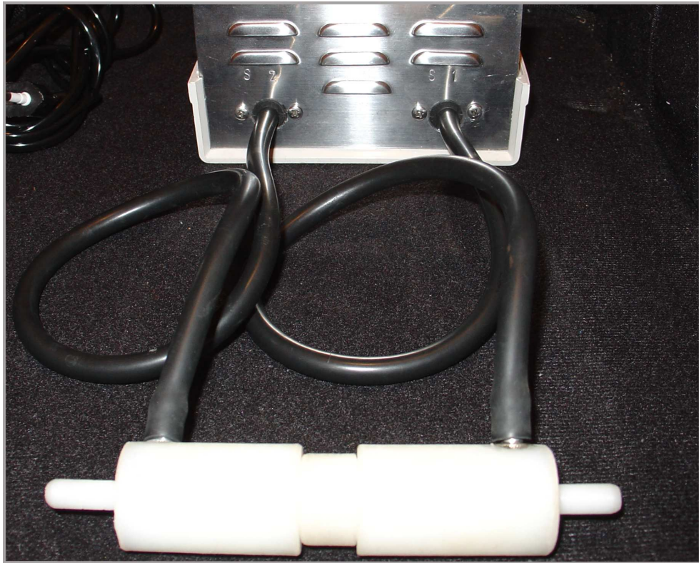
Figure D.3 Connection of the airway resistor to the analyzer
