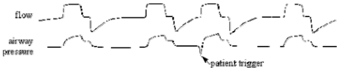
Figure 2.6 Example waveform of the pressure and flow relationship in a volume controlled mode [10]
