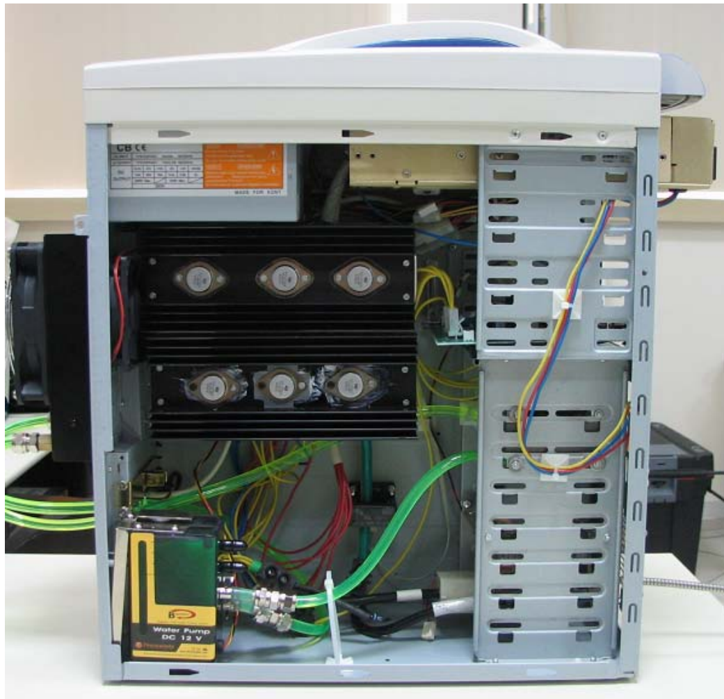
Figure 4.18 Side view of PC case after installation.
