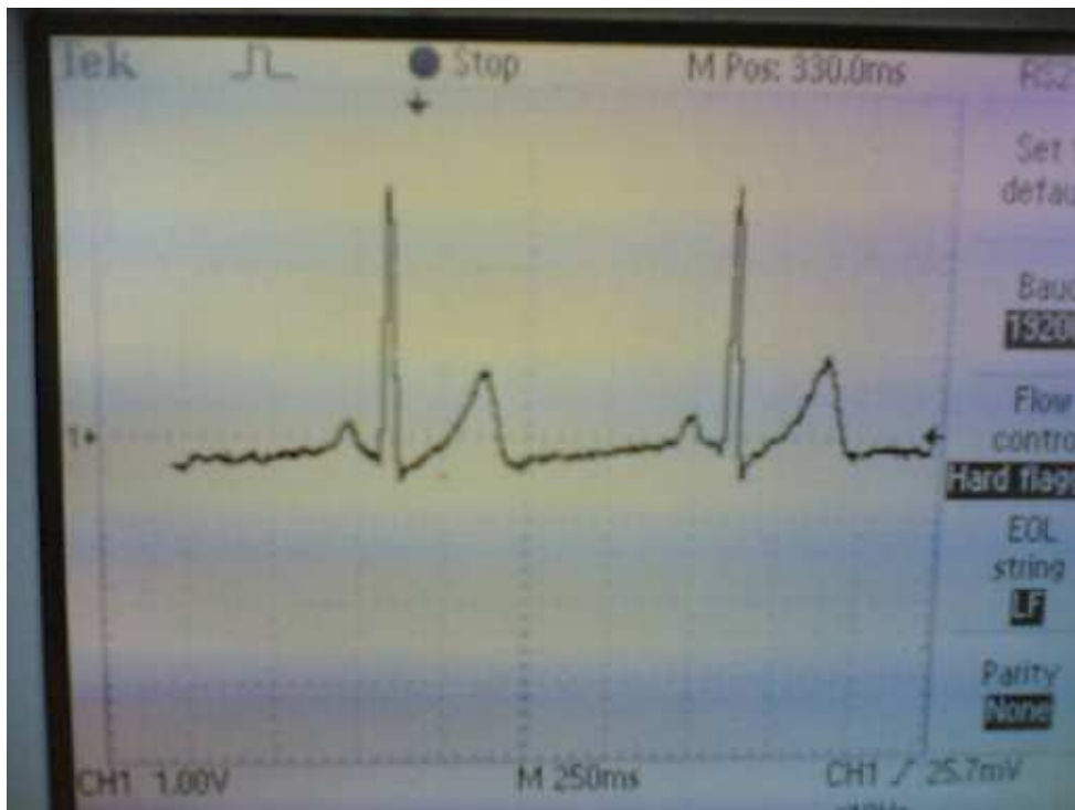
Figure 3.16 A snapshot of the ECG data viewed on oscilloscope screen
