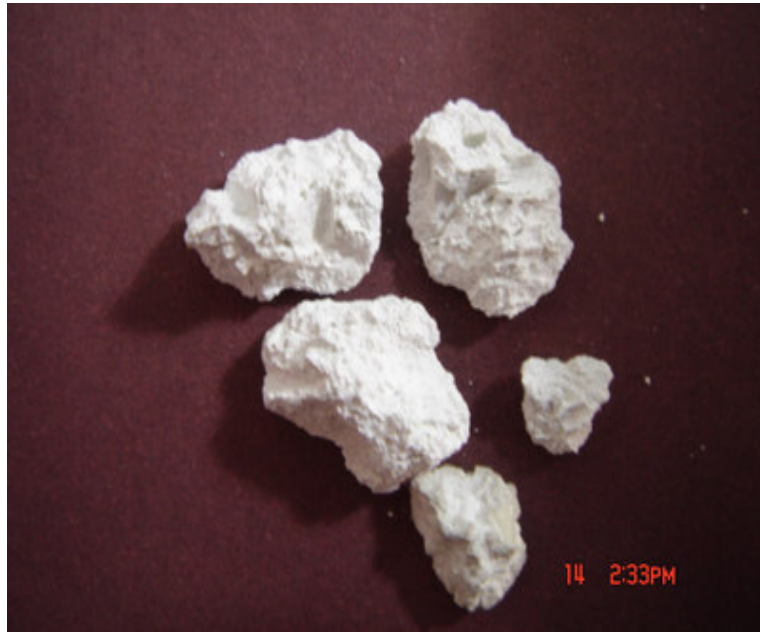
Figure 12.2 The pieces of broken specimen due to the high pace of temperature increase and high thermal gradient within the specimen
