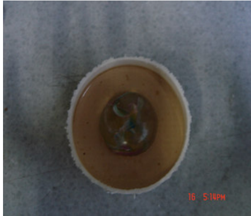
Figure 11.4 Embedded marble in the gypsum plaster
