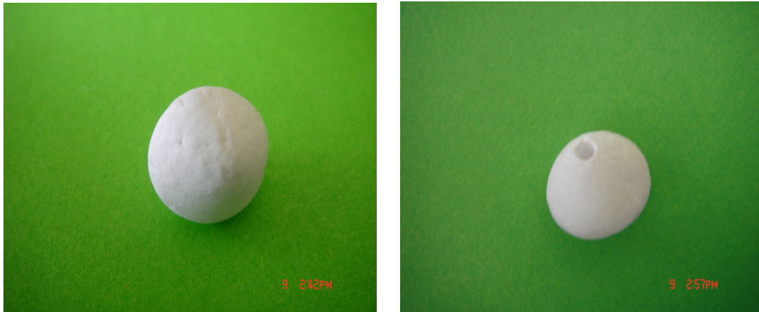
Figure 12.3 a ) Sintered HAp sample without any defect b) A little hole was drilled by a hand drill on the sample
