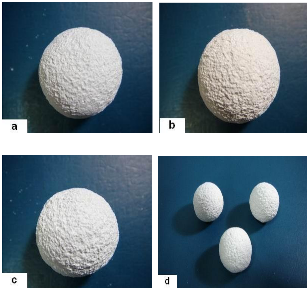
Figure 12.5 a,b,c) Image of a %30, %40 and %45 naphthalene added specimen implants respectively d) All three specimen implants are together
