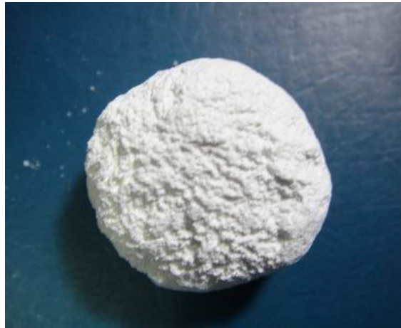
Figure 12.6 %60 naphthalene added, deformed specimen implant sintered at 1200 °C for 3 hours
