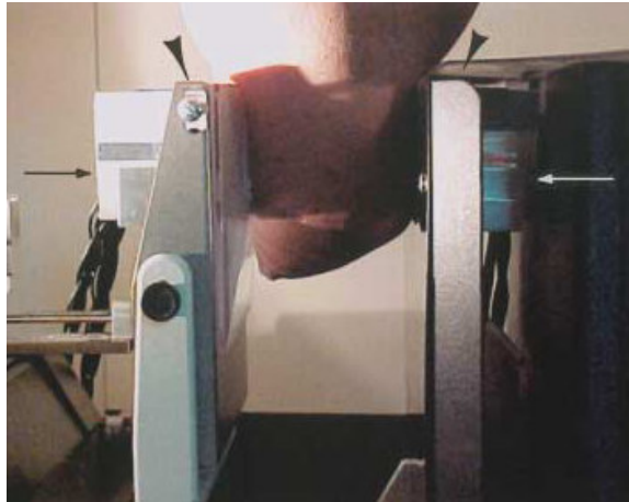
Figure 3.13 Geometry for PEM detector by Adler et al. After PEM image acquisition, X-ray-guided biopsy can proceed without releasing breast compression [44].
