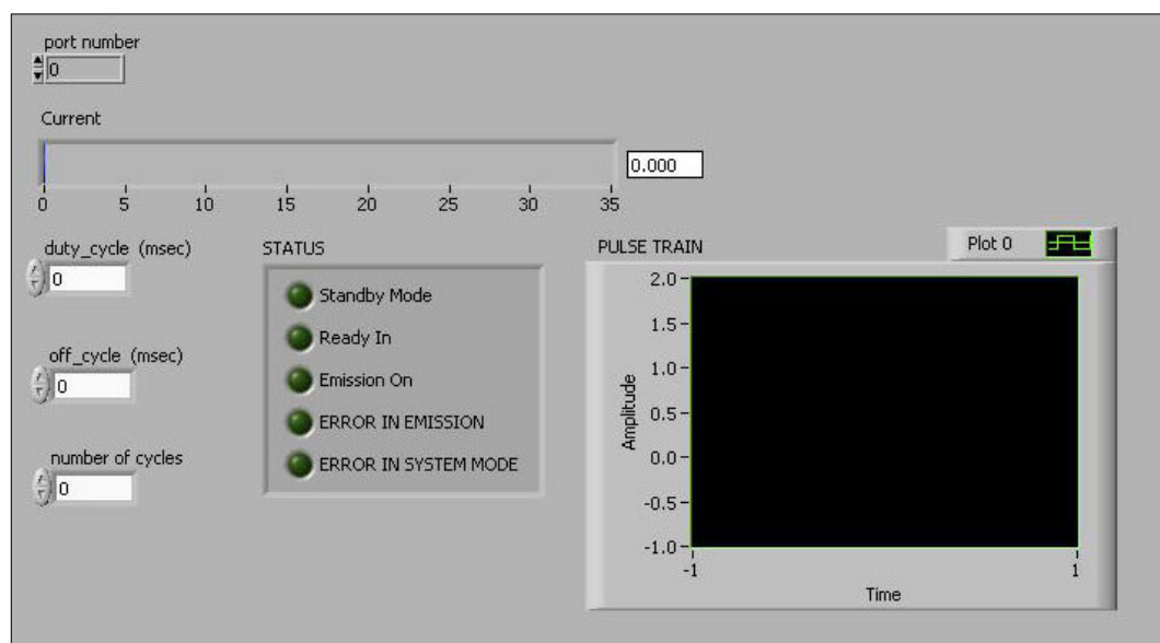
Figure 3.2 Laser interface. Laser parameters (duty cycle, off cycle, number of cycles) were adjusted by using this interface. To determine the power levels, previously defined current values were used.
