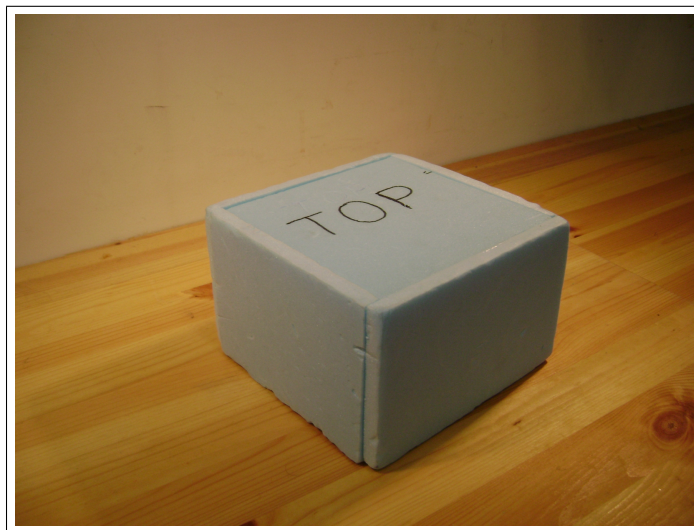
Figure 4.1 Rectangular gel phantom with heat insulation
