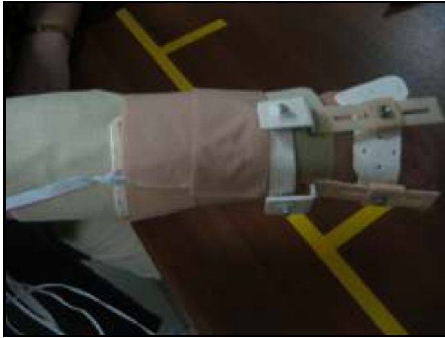
Figure 3.43 The positioning of the electrogoniometer on the forearm_1
