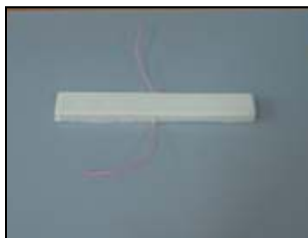
Figure 3.8 The hardened silicon containing PVC sheet with strain-gauge
