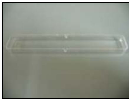
Figure 3.7 The plastic mold used in the construction of the sensor
