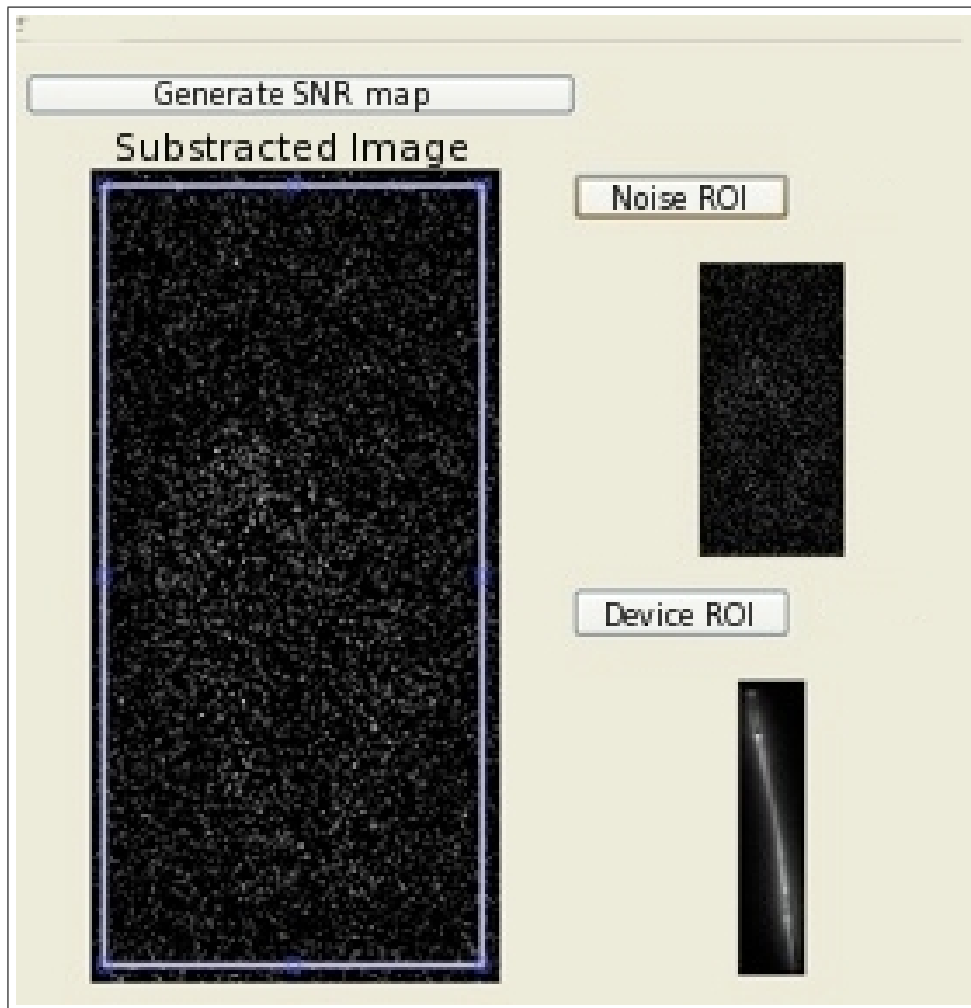
Figure 3.6 (left) The entire subtracted image was used as noise ROI. (right bottom) The active guidewire device region selected as device signal.
