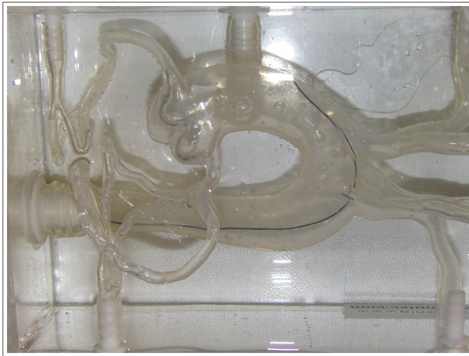
Figure 2.9 The silicon aortic arch model filled with saline solution. The guidewire was placed inside the model for in vitro visibility test under MRI.
