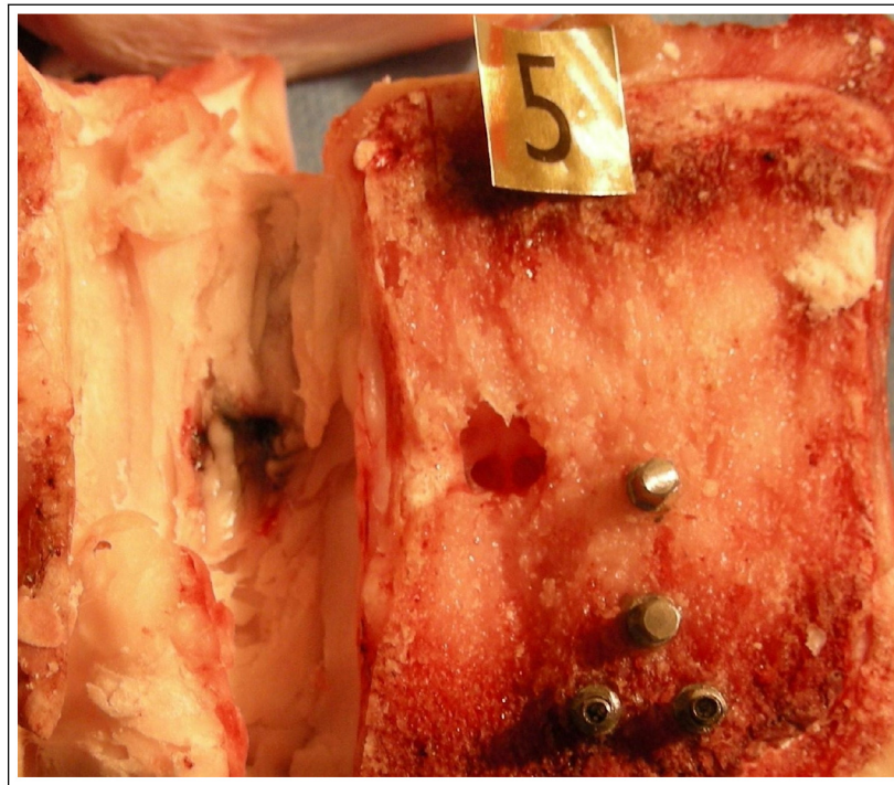
Figure 13.6 Bovine spinal bone sample 5, implants are placed by torque control.
