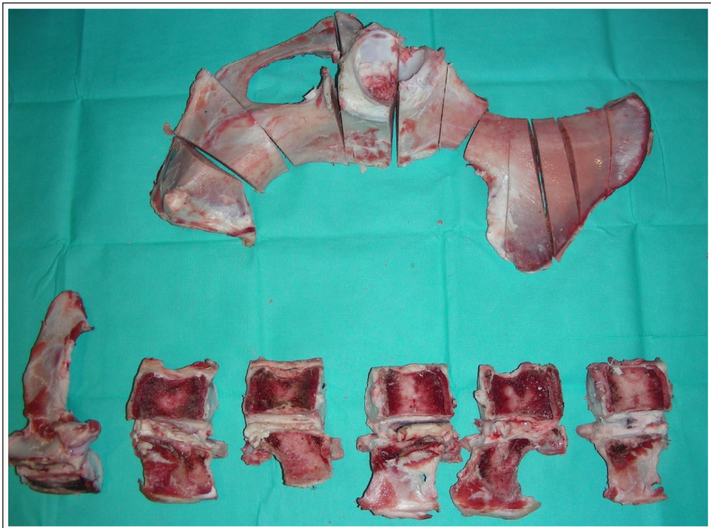
Figure 13.1 Bovine iliac and spinal bone pieces cut into segments for bone testing.
