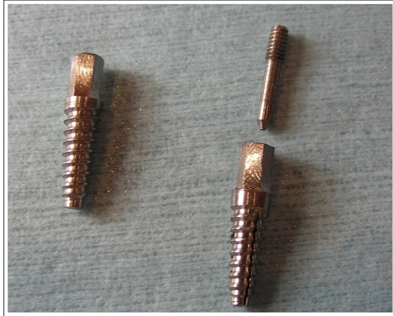
Figure 12.14 Manufactured control implant (left) and developed implant design (right).
