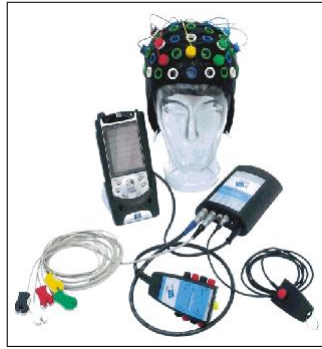
Figure 2.9 G.tec Company EEG Amplifier: For a variety of BCI technologies, g.tec is a source of one of the best head caps used in the field involving wet electrode recordings[32].
