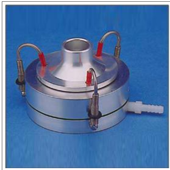
Figure 3.3 Single-Stage Impact Sampler.[3]
