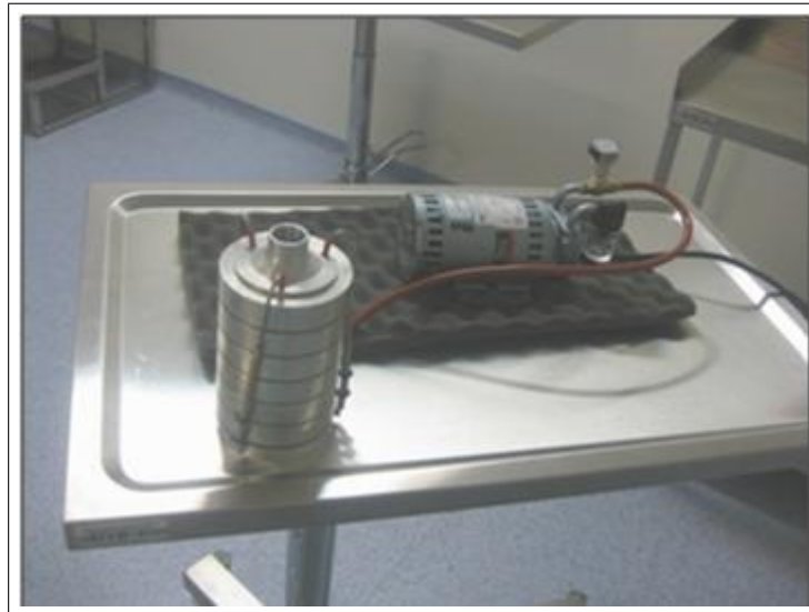
Figure 4.5 New-Star Andersen Six-Stage Viable Counter used in the experiments.
