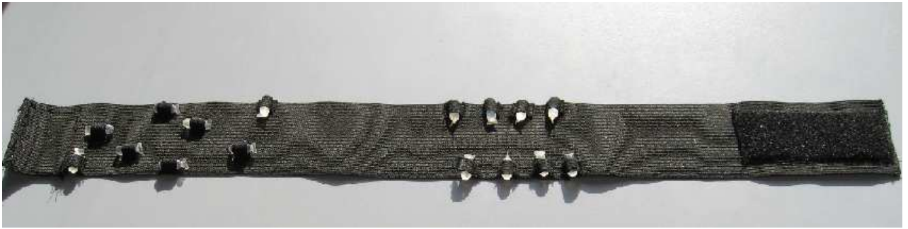
Figure 2.1 Multi-modality marker belt used in XFM study. Markers are located on the belt with specific pattern for the ease of segmentation of XF images. (Taken from [7])
