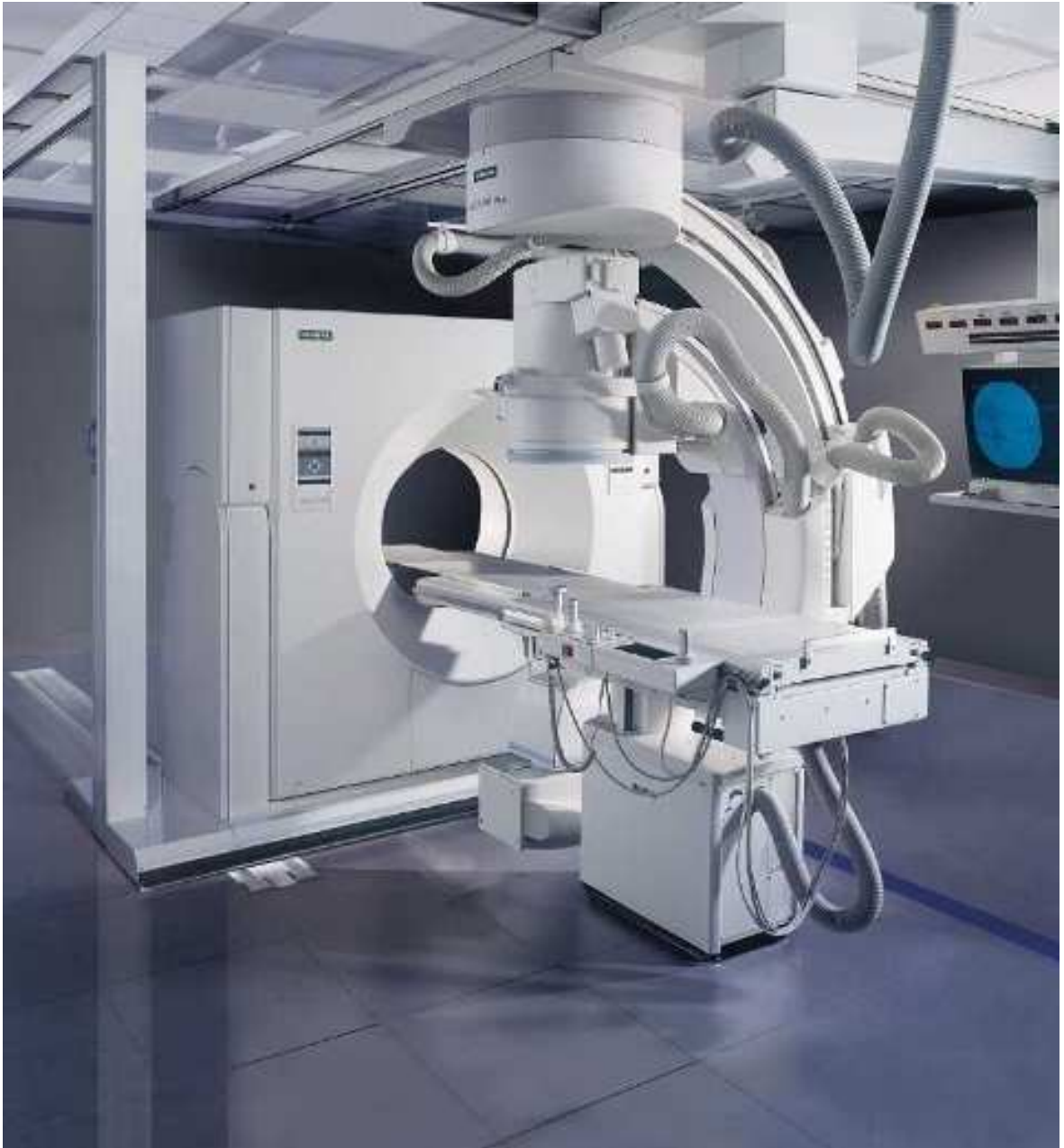
Figure 1.1 Combination of a 16 slice CT, and X-ray Fluoroscopy. Advantage of CT on acquisition of cross-sectional images of the body which could be combined to give the 3D volume, and practical use of XF combined together. [10]
