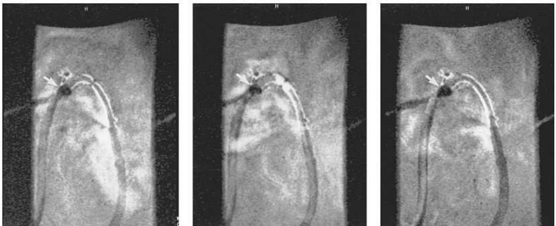
Figure 1.3 In vitro model. Sagittal view (white arrows in all three panels: artifact of the marker on the tip of the nitinol guidewire). Left: Creation of a dilatable stenosis on a porcine segment of aortic arch connected to the plastic tubes. Middle: Angioplasty by a fully pressurized balloon. Right: Complete resolution of the stenosis after dilatation. [14]
