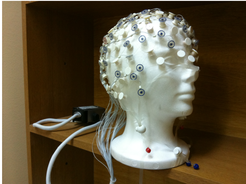
Figure 3.2 64 channel EEG cap with sponge electrodes.
