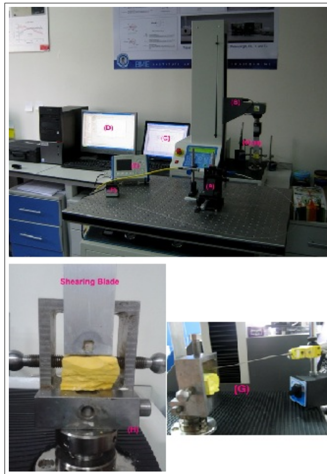
Figure 3.7 (A) 1940- nm Thulium Fiber Laser , (B) Universal testing machine (Lloyd, LF Plus, UK) , (C) Computer for collecting and recording data from the thermocouple , (D) Computer that is connected to universal testing machine for controlling and collecting and recording data , (E) Monitor and controller of Powermeter (Newport, Model 1918-C) , (F) Sensitive measuring head of powermeter, (G) K-type thermocouple (OMEGA, OM-CP-0CTTEMP, UK), (H) Shearing Blade.
