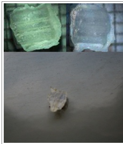
Figure 4.6 Indication of Remnant Adhesive Material On the Bracket Base.
