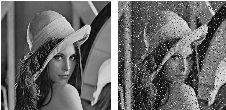
Figure 2.18 Left image is original lena image. The image on the right shows salt and pepper noise on the lena image.
