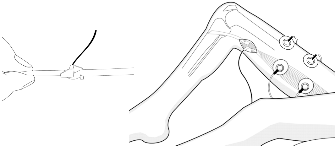
Figure 4.1 Usage of buckle force transducer and stimulation electrodes. Illustrations of how (A) the buckle force transducer is mounted over tendon strips, and (B) the skin electrodes are mounted over the GRA and VM muscles are shown.
