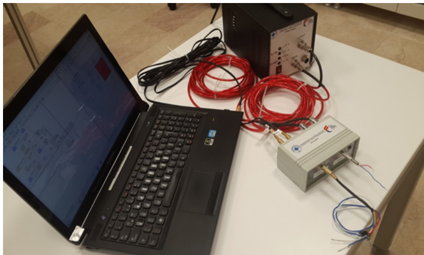
Figure A.2 The stimulator is shown next to the laptop. The power supply is below the oscilloscope.
