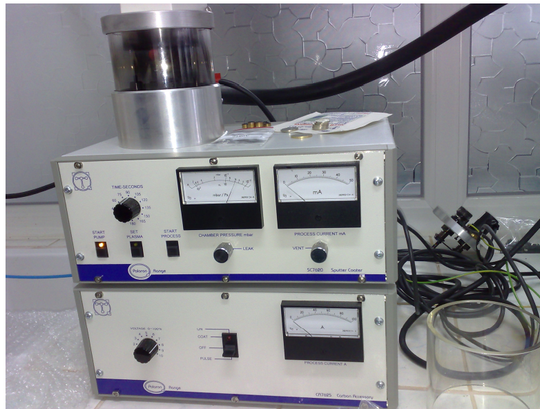
Figure 2.5.2.2 Polaron SC7620 SEM sputter coater with CA7625 carbon accessory.
