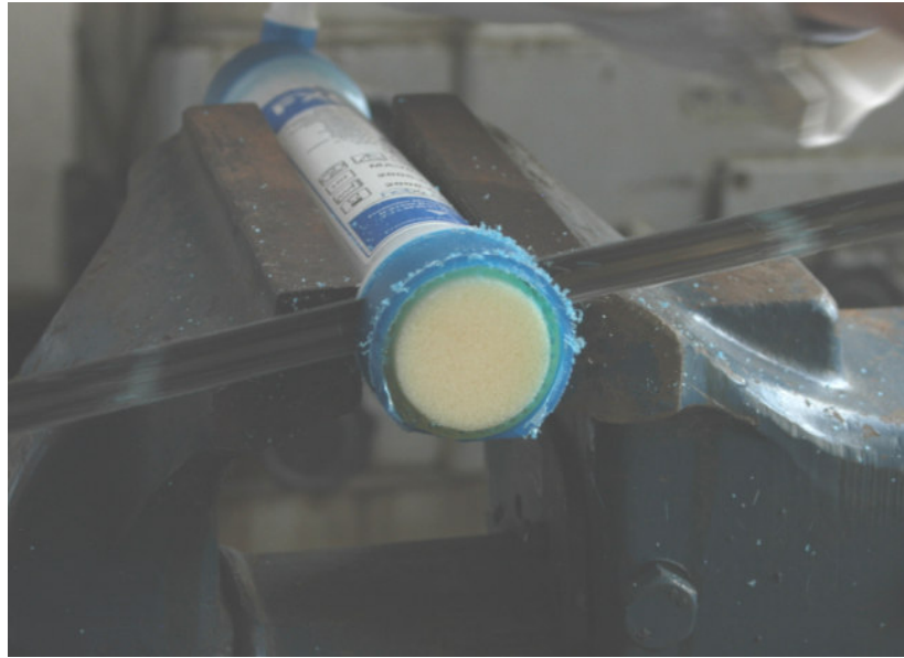
Figure 2.1.2.2 The picture of cutting the hemodialyzer which was mounted in a vise (Step – 2 in Figure 2.1.2.1).
