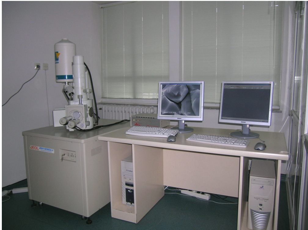
Figure 2.5.2.1 JEOL JSM-6060LV scanning electron microscope.
