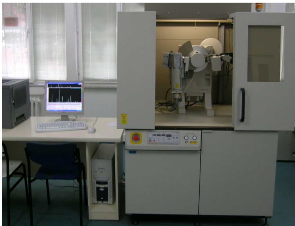
Figure 2.6.2.1 Rigaku D-Max 2200 X-ray diffractometer.
