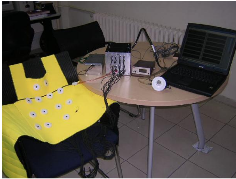
Figure 2.1 The components of the DAQ System, i.e. 14 air-coupled microphones, a box containing amplifiers and filters, a flow-meter and DAQ Card embedded in a laptop computer.
