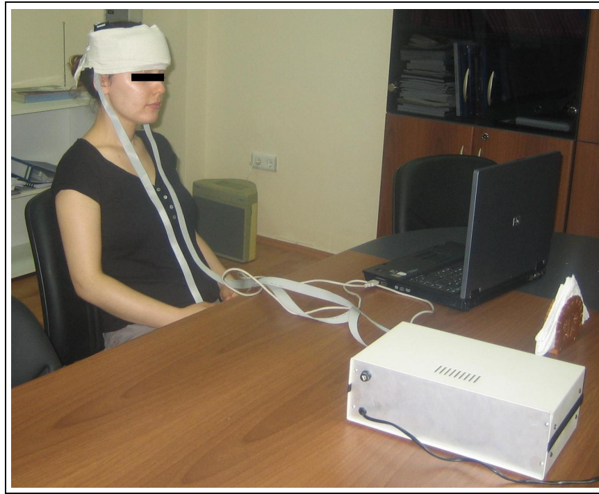
Figure 3.2 MA task data taking with functional optical imager, NIROXCOPE 301
