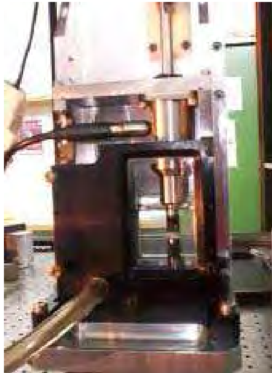
Figure 3.3 Mechanical testing apparatus. A stainless steel rod, attached to a sub-micrometer high precision DC motor and controller and coupled with a water-proof load-cell is used as an upper compression anvil, while the lower anvil is stationary. In order to maintain the physiological viscoelastic properties of bone samples, a specially made water cell is mounted on the mechanical compression apparatus orthogonal to the optical axis of the CCD detector array. A custom-built positioning rack with precision positioning rails prevents any horizontal displacements of the water cell.
