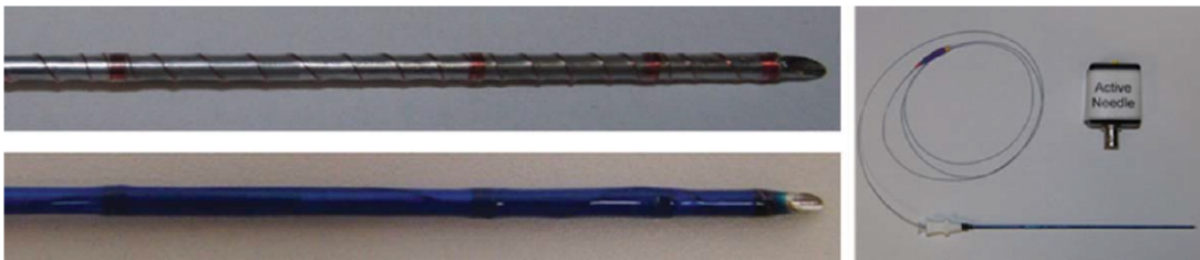
Figure 2.8 Active needle with close-up of tip uncovered (top) and covered (bottom) [3].
