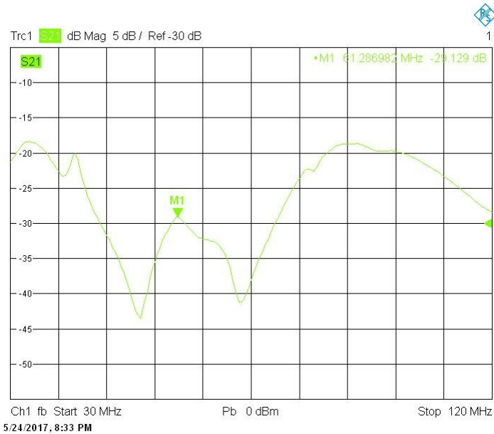
Figure 5.10 S_{21} results of the monopole antennas in the phantom (The Green marker shows that S_{21} is -29 dB at 61 MHz).
