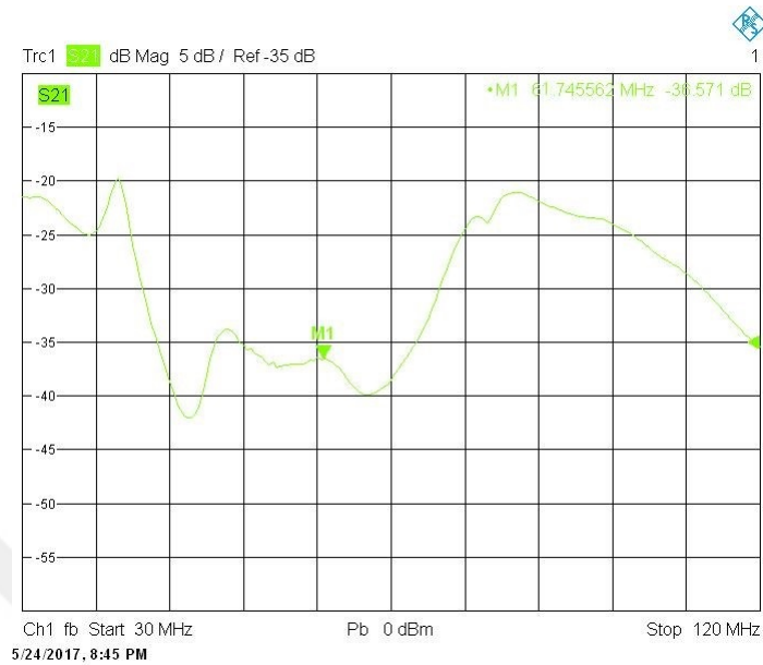
Figure 5.13 S_{21} results of the monopole antennas in the phantom with a conductive silver ink shielding planar geometry (The Green marker shows that S_{21} is -36.6 dB at 61 MHz).
