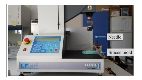
Figure 2.10 Stiffness testing mechanism (LLOYD instruments, LF Plus digital testing machine).
