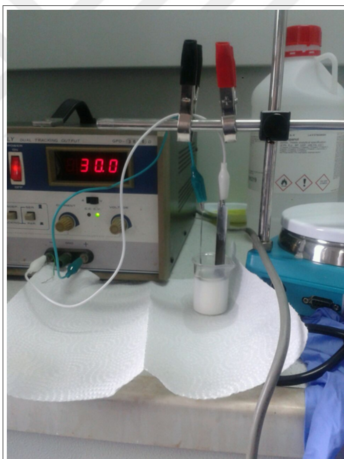
Figure 3.3 Experimental setup for EPD
