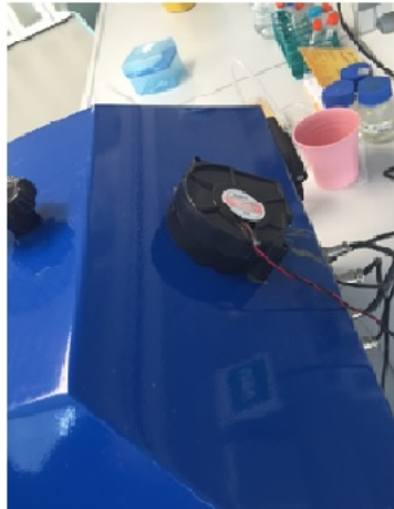
Figure 2.6: A fan was placed on the back face of the cap and vent holes were punched at the bottom of the box.
