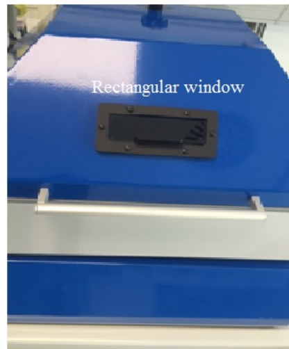
Figure 2.4: A rectangular window was placed in front of the pyramidal cap to visualize gel with naked eye during the run.
