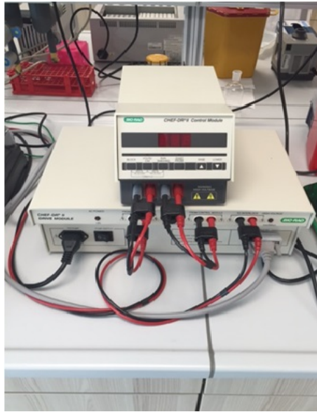
Figure 1.8: High Voltage Power Supply and Switch Unit
